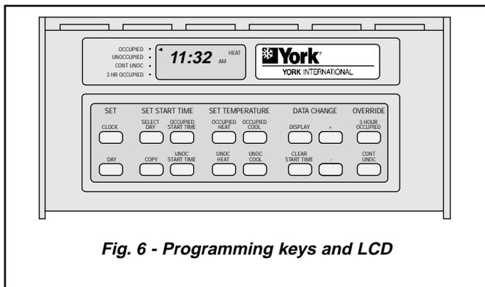
Fig. 6 - Programming keys and LCD
