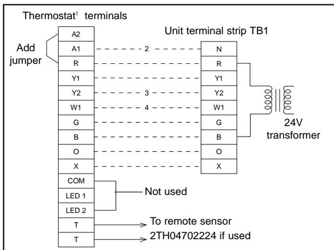
1. Electronic programmable thermostat 2ET04700324 with subbase for both manual and automatic changeover.
