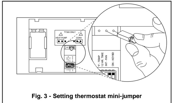
Fig. 3 - Setting thermostat mini-jumper
