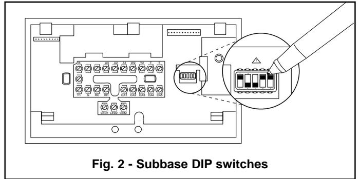
Fig. 2 - Subbase DIP switches
